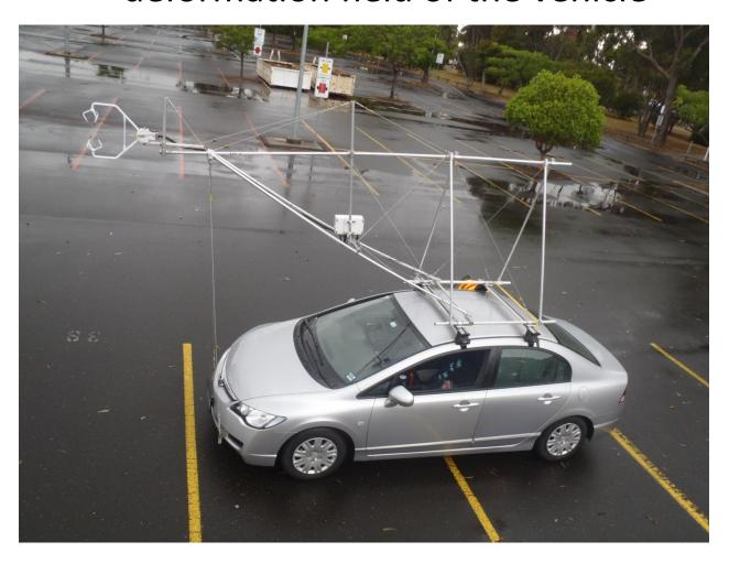
A CSAT3 with a fine wire thermocouple measures the 3D wind and fast response temperature. To measure the location of these measurements we use a low-cost GPS-enhanced Attitude and Heading Reference System (AHRS) IG-500N. It is fundamentally a miniature Inertial Navigation System with performance similar to those systems used in aircraft. It measures the 3D orientation, position and velocity at 100 Hz.
