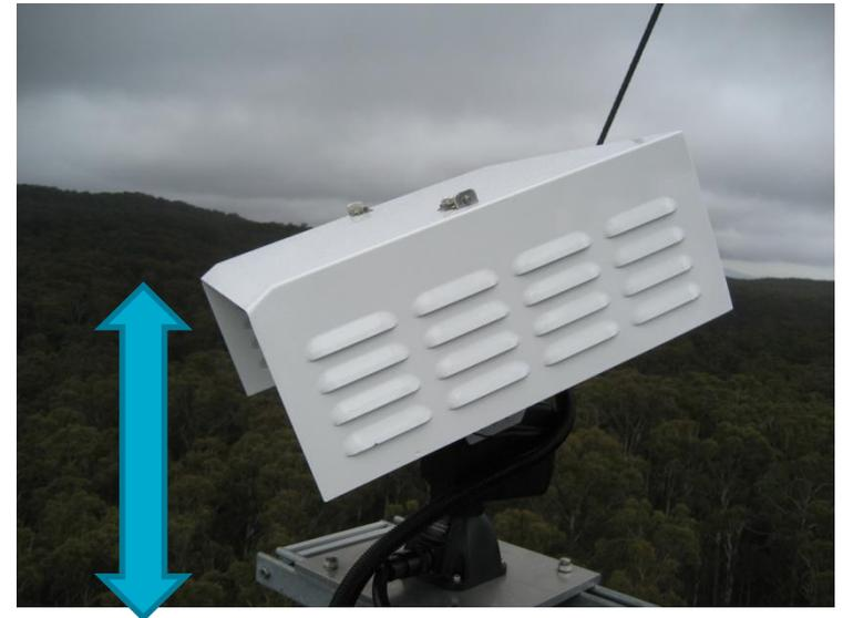
White box is a radiation shield to minimise heat input from the sun. Unit is mounted on rails for ease of access. PC etc. is mounted in another box nearby on the tower.
