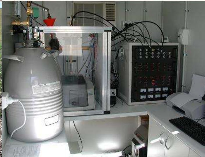
Air from chamber head space circulated through Fourier Transform Infrared Spectrometer (courtesy of UoW) and rate of increase in CO 2 concentration measured (along with CH 4 and N 2 O emissions)
